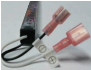
ILT-10-EP-1-LED End Prep for 1010 3" Black and White 18ga wire connector lead with Male and Female spade connectors on one end and a dead end cap on the other end. Polarity is "+" on White and "-" on Black.
