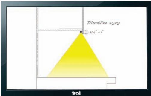
Under Cabinet / Task Lighting
